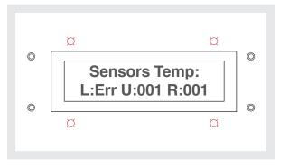
**Troubleshoot:** Ensure power is switched off to the controller then check the sensor cable condition for any cuts or defects in the cable. If any defects in cable is found, please contact Solargain service department on 1300 73 93 55. Do not try to repair the cable as this will void warranty.
